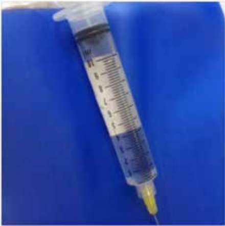
Figure 3. With graduated syringes it is easy to control the flow rate: aim for about 1 ml over 15 seconds.
